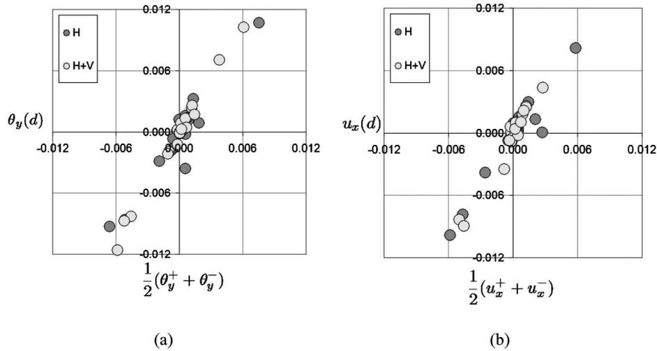
Fig. 14. Correlations between difference of extreme values versus residual values for (a) rotation and (b) horizontal displacements of the foundation
