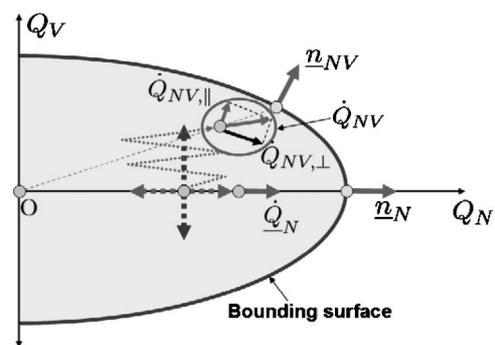
**Fig. 9. Schematic representation of typical stress paths in the space of the generalized forces (plane  $Q_N$ - $Q_V$ )**
