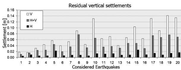
**Fig. 7. Residual settlements of the foundation for the considered records and for the three cases of analyses**
