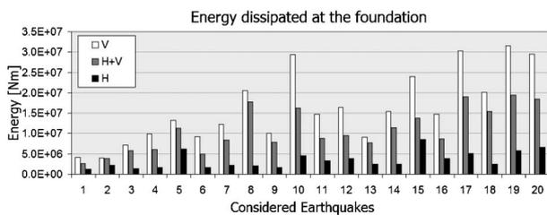
**Fig. 8. Total dissipated energy at the foundation for the considered records and for the three cases of analyses**
