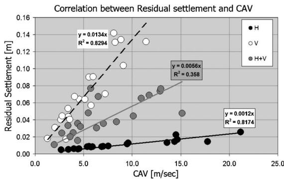
Fig. 10. Correlation between CAV and residual settlements of the foundation
