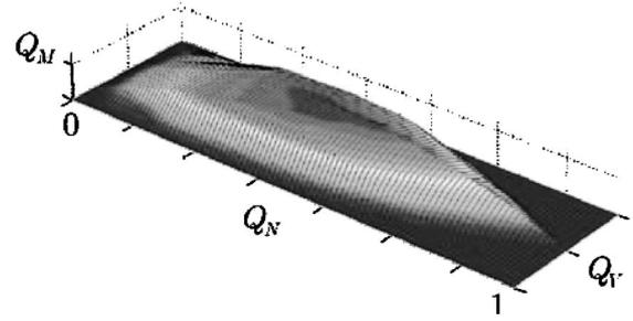
Fig. 4. Approximation from outside of the surface of ultimate loads of a circular footing on a homogeneous cohesive soil (cf. Chatzigos et al., 2007). Uplift is allowed at the soil-footing interface
