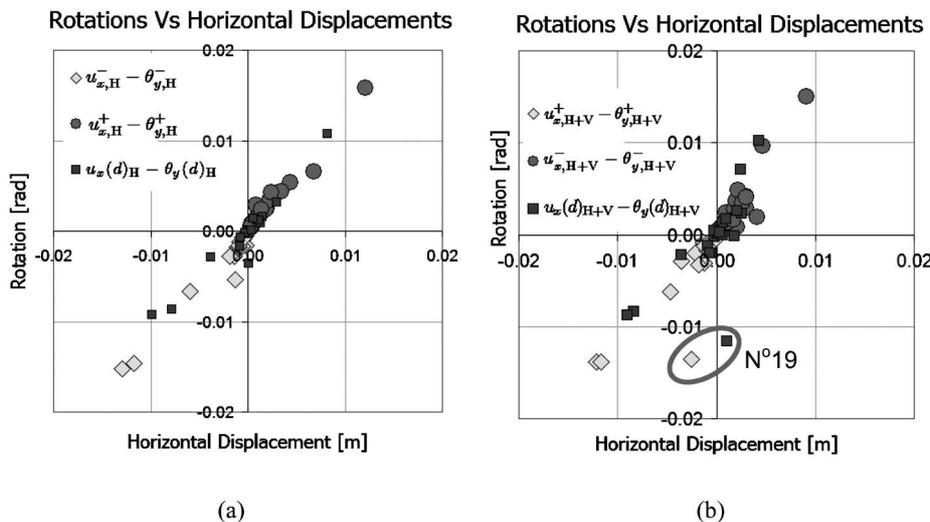
Fig. 13. Characteristic rotations of the foundation plotted versus the corresponding horizontal displacements: (a) Analyses H and (b) Analyses H + V
