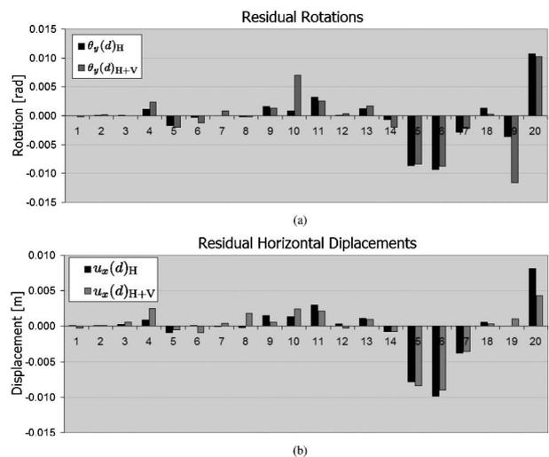
Fig. 11. (a) Residual rotations and (b) Residual horizontal displacements of the foundation
