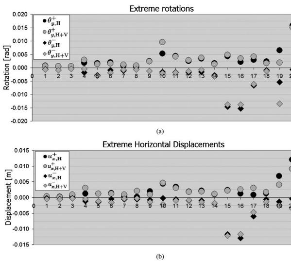
Fig. 12. (a) Extreme values of rotations and (b) Extreme values of horizontal displacements of the foundation
