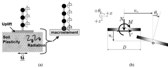
Fig. 1. (a) Definition of the concept of macro-element and (b) Forces and corresponding kinematic parameters for a shallow perfectly rigid footing
