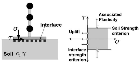
**Fig. 2. Examined configuration for soil and soil-footing interface. The soil strength criterion induces in the macroelement scale the non-linear mechanism of soil plasticity. Similarly, the interface criterion induces in the macroelement the non-linear mechanism of uplift. Note that plasticity is dissipative while uplift takes place with zero dissipation**
