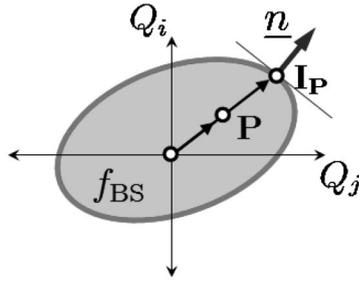
Fig. 3. Bounding surface and radial mapping rule for the definition of the image point
