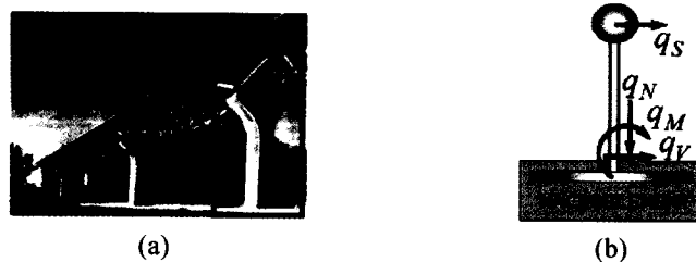
Fig. X.4 (a) Typical bridge pylon and (b) simplified model for non-linear dynamic analyses with macroelement.
