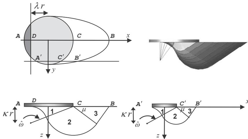
Figure 5. Shear-rotational virtual failure mechanism
