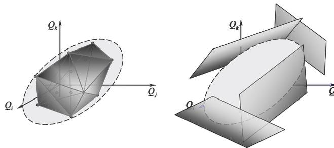
Figure 1. Internal and external approaches of the domain of potentially safe loads
