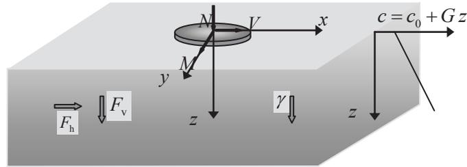
Figure 2. Circular shallow foundation under seismic loading on a purely cohesive soil
