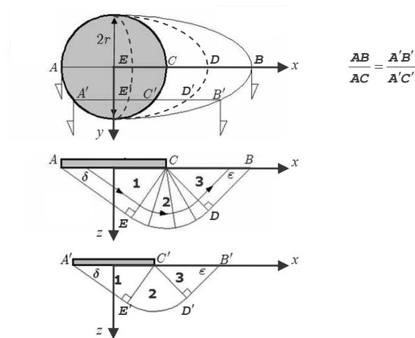
Figure 3. Translational virtual failure mechanism
