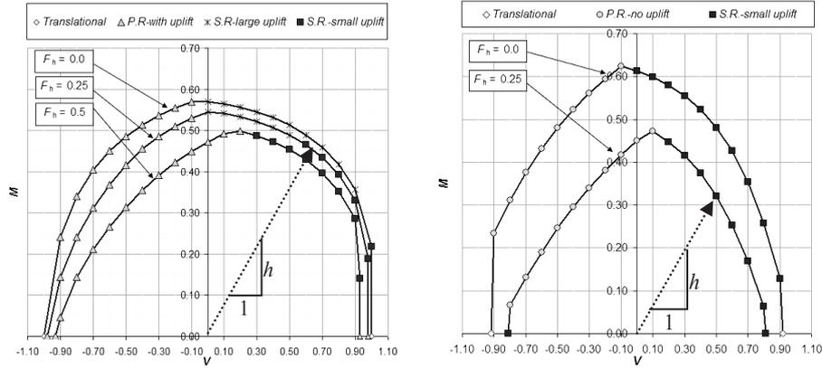
Figure 7. Tresca criterion with zero tension “cut-off”: ( $N=const., V, M, F_h$ ) Interaction diagram for  $k=0$ ,  $N_{max}^0 / N > 3$  and  $N_{max}^0 / N > 3/2$ ; ultimate loading paths for  $F_h = 0,25$  in a SDOF superstructure
