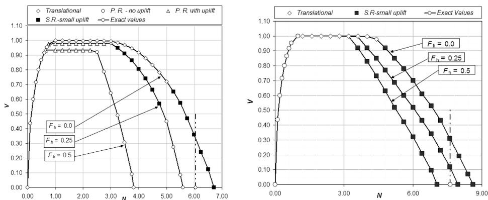
Figure 6. Tresca criterion with zero tension “cut-off”: Interaction diagram  $(N, V, M = 0, F_h)$  for  $k = 0$  and  $k = 1$
