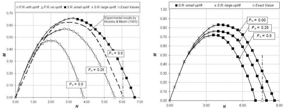
Figure 7. Tresca criterion with zero tension “cut-off”: Interaction diagram ( $N, V=0, M, F_h$ ) for  $k=0$  &  $k=1$ , and experimental results by Houlsby & Martin [8]
