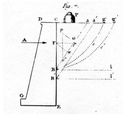
**Figure 5.** Stability analysis of a retaining wall from Coulomb's *Essay*.
