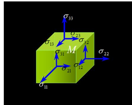
**Figure 6.** Cauchy's Memoir *On pressures and tensions acting on three mutually orthogonal planes at a given point of a solid body*. Presentation of the 9 components of the surface density of forces.
