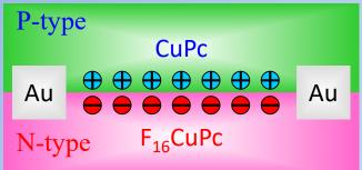
• Free holes and electrons in CuPc and  $F_{16}$ CuPc can be easily driven along the interface by an electric field applied across the drain and source electrodes
