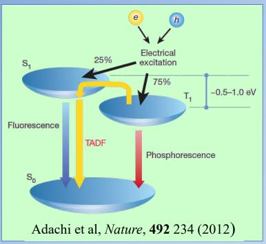
Thermally activated delayed fluorescence (TADF).
