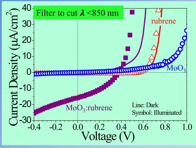
1<sup>st</sup> IR solar cell based on CTC absorption.
